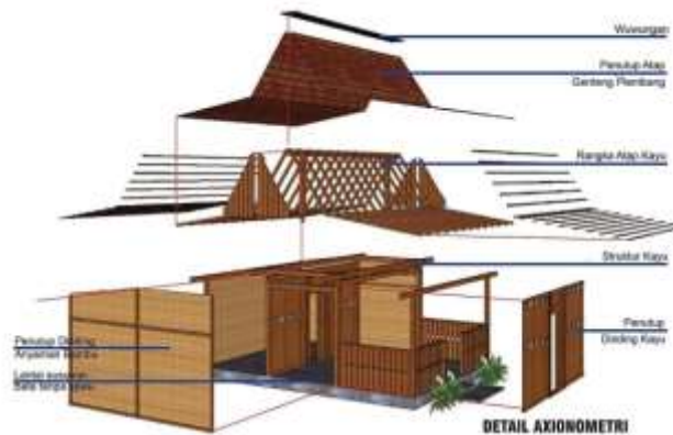
Figure 4. Material structure of the Osing traditional house (Source: Perbup Banyuwangi No.11 of 2019, about Osing architecture)
